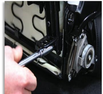
Attach return spring as shown in illustration (2A), (2B) between the two sprung points. This will allow the seats locking mechanism to activate once the seat is slid to the desired position of choice
